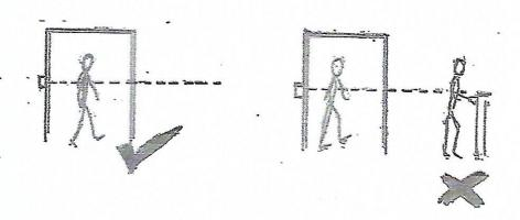
Position approximately 1.5 metres from ground level and fix in place using either the wall mount hook fixer or the side mount VHB fixing tape.
