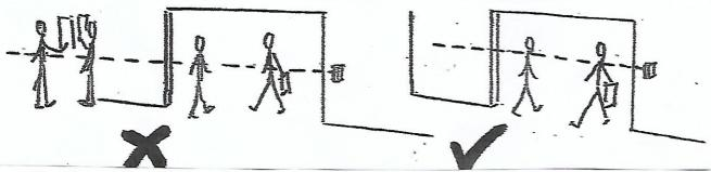
The beam length has been set at its mid point (around 5 metres) and after testing should this need to be adjusted locate the range adjustment pot
