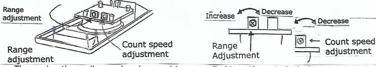
Then using the mall cross head screwdriver supplied turn the pot clockwise to increase range and anti clockwise to decrease. NOTE the pot is very delicate and will not turn beyond ¾ of the dial so not force it. Adjust and test again.
