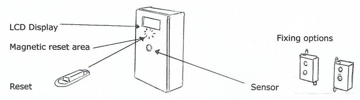
The LTB-7 footfall counter provides a single sided wall mounted solution for most entrances.
